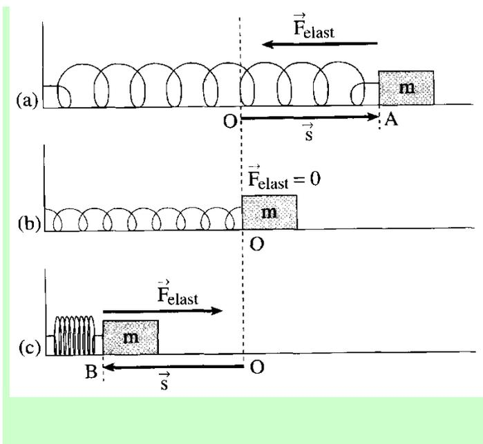
$$T = \frac{2\pi}{\omega} = 2\pi\sqrt{\frac{m}{k}} = 2\pi\sqrt{\frac{m x}{F}} = 2\pi\sqrt{\frac{x}{a_x}}$$
