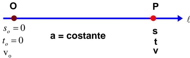
$$s = v_0 \cdot t + \frac{1}{2} a t^2 \quad v = v_0 + a \cdot t \quad a = \frac{v - v_0}{t} \quad t = \frac{v - v_0}{a} \quad a = \frac{2(s - v_0 t)}{t^2}$$
